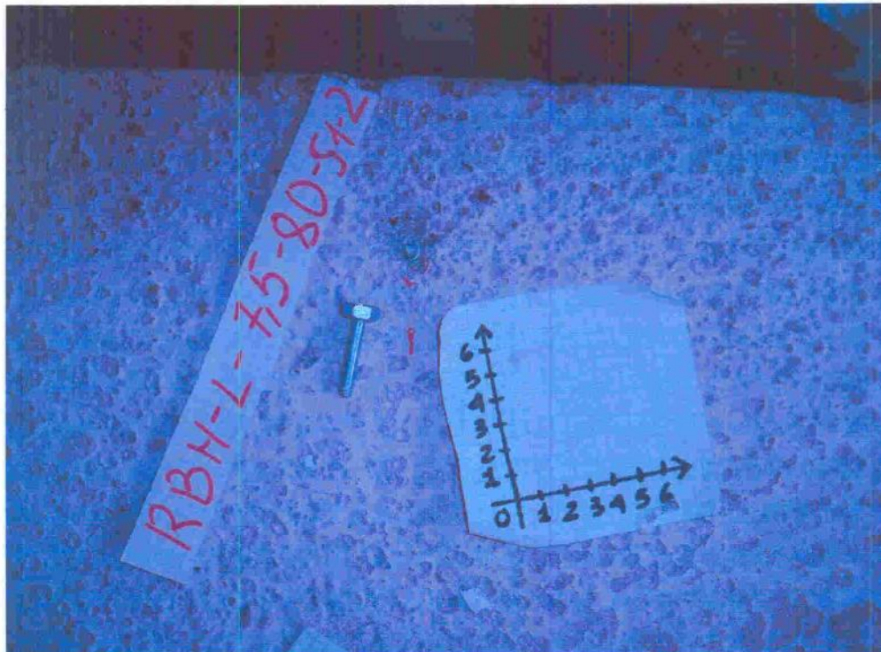
Fig. 6: Shear tests M7.5 - S1-2: steel failure.
